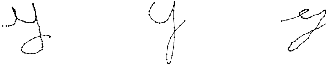
Figure 2.1: Differences in sample point spacings for handwritten characters. Each dot indicates the location of a sample point.
