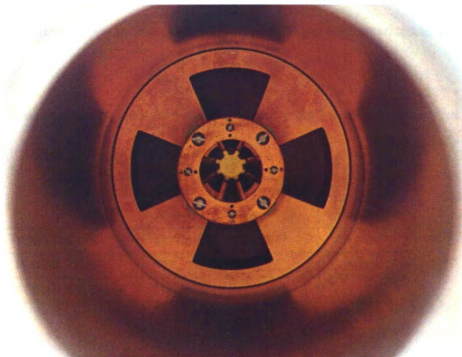
Figure 79. A view of the fully assembled rf cavity looking into the extraction end. The 8 tapered magnetron vanes of the acceleration section can be seen inside the ID of the exit mounting ring.
