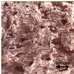
Figure 5 SEM micrograph of the outer surface of 65/35 P(dl)A/PGA/Fe implant containing 25 vol. % Fe, 50x
