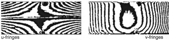
Figure 4.6.- Moire fringe patterns of various joining subjected to four point bending: (a) 2S3 (90N) (S for stitching and 3 for three stitches per 50 mm), (b) 2S3 (200 N) , (c) 2S5 (S for stitching and 5 for 5-by-2 stitching pattern), and (d) 2BS3 (B for bonding, S for stitching and 3 for three stitches per 50 mm)
