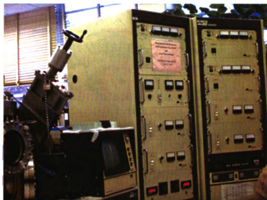
Figure 2.1 Front views of the MSU sputtering system with four dc-triode guns and a magnetron gun capability, including the related power supply and the residual gas analyzer.
