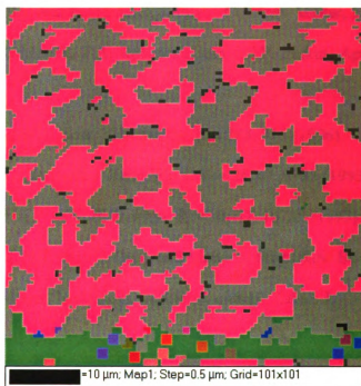
Figure 5.A.3. Orientation maps of 200 nm epitaxial Ag films grown on epitaxial Nb at substrate temperature of 350°C. The green areas are unsolved points (loss of EBSD signal).
