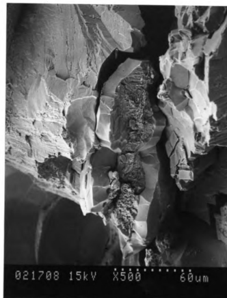
Figure 4.29. Reaction Zone in a SiC Particle Reinforced \gamma -Ni 3 Al Matrix Composite with Aluminum Nitride Film Deposited at 793 K as a Diffusion Barrier.
