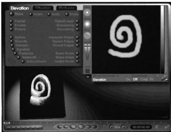
Figure 3. Example of Bryce3D “terrain” generated from a grayscale image.
