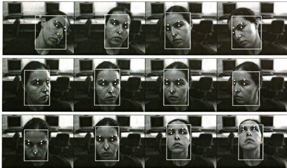
Figure 3.12: Results of eyes-nose detection for various roll, pan and tilt angles. The white rectangle shows face boundaries, and the white dots show the locations of the eyes, eyebrows and tip of the nose.
