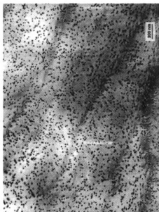
Figure 7.11 TEM image of columnar defects in YBCO, looking along the defect direction. Defects were created by 1.3 GeV uranium ions.
