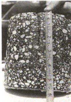
Figure 3-5. Core showing surface-initiated longitudinal wheel path cracks (Myers et al., 1998)
