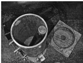
Fig. 2.2 Cylindrical mold used for freeze-thaw test specimens
