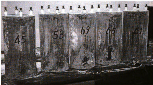
Fig. 2.9 Severely corroded specimens prior to patching
