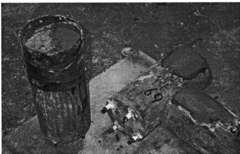
Fig. 2.10 Patching of the severely corroded specimens
