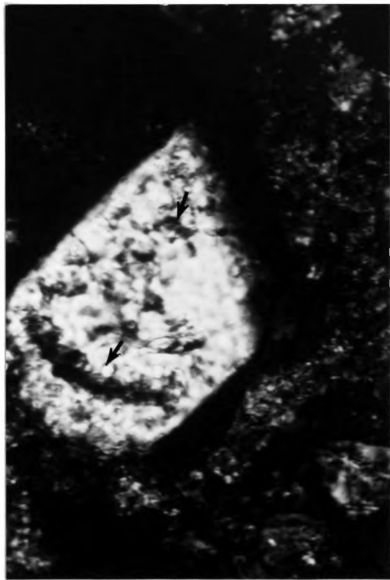
Figure 15. Cathodoluminescent image of Serro Domi sample exhibiting inclusions and dissolution. Left arrow points to an inclusion. Right arrow points to dissolution (1 inch = 50 microns).
