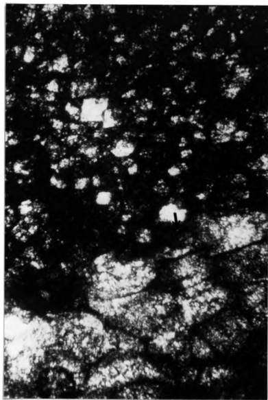
Figure 26. Partially crossed polar view of Saluda packstone. Arrow points to fossil fragment (1 inch = 200 microns).
