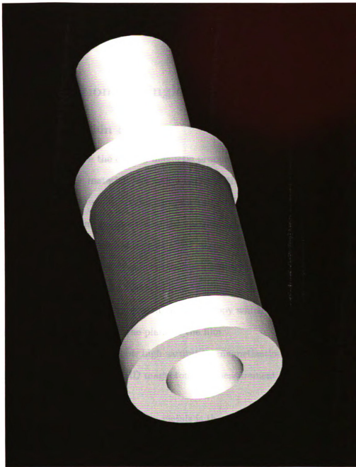
Figure 3.10: Representation of the homemade solenoid magnet used in the switching field characterization experiments. The inner bore of the magnet is 0.5in, and the overall length is 3.0in.
