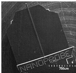
Figure 3.4: An SEM image of an AFM tip.
