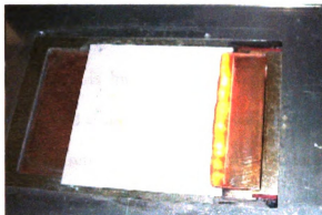
Figure 13a. Uniform, flat flame front in MSU Flame Rig.
