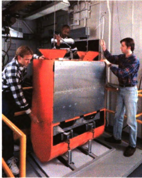
Figure 8. Drag shield in 2.2 Second Drop Tower.
