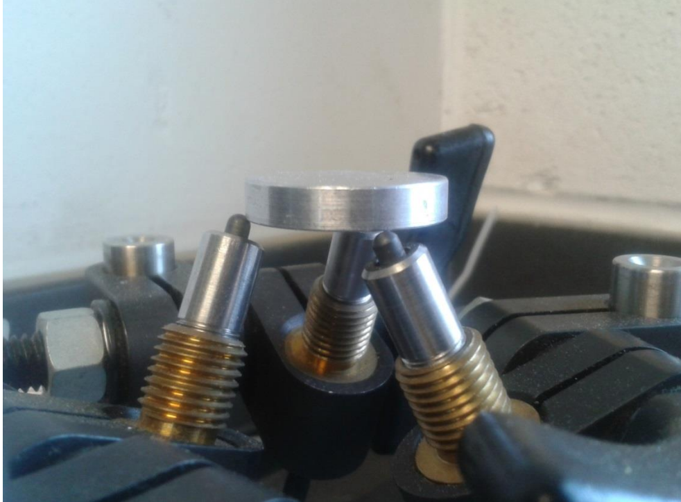
Figure 2.3.1 An aluminum sample mounted to the three transducer setup. Notice in the image how the transducers are on the edge of the specimen. The transducers are rounded so the contact area is very small. Aluminum was not studied here, but the large specimen makes a clear visual.
