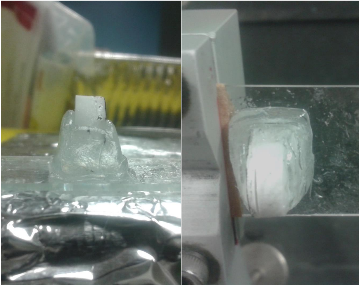
Figure 2.2.1 The LLZO billet being prepared for cutting. The left image shows the billet being affixed to a glass slide with thermoplastic covering more than half of the specimen to prevent chipping. Some minor chipping can be seen, as that was how the specimen was received. The image on the right shows the glass slide mounted to the cutting arm of the slow speed diamond saw. A cut that had been started can be seen on the left side of the billet.
