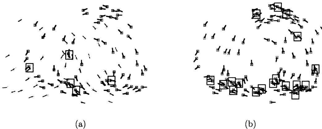
Figure 2.4: Minutiae matching for (a) twin-nontwin (matching of Figures 2.3(e) and 2.3(f), matching score = 3 on a scale of 0-999) and (b) twin-twin (matching of Figures 2.3(d) and Figure 2.3(e), matching score = 38 on a scale of 0-999). The “matched” minutiae pairs are shown by bounding boxes.
