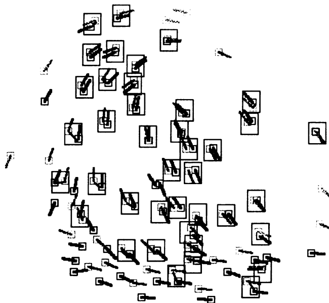
Figure 2.5: Minutiae matching for two impressions of the same finger shown in Figures 2.2(a) and 2.2(b) (matching score = 487 on a scale of 0-999). The “matched” minutiae pairs are shown by bounding boxes.
