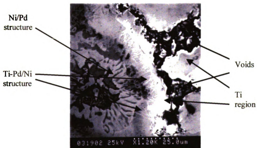
Figure 3-6 SEM photomicrograph at 1200 X of the Ti 53.5/Pd 25/Ni 21.5 at. % Target
