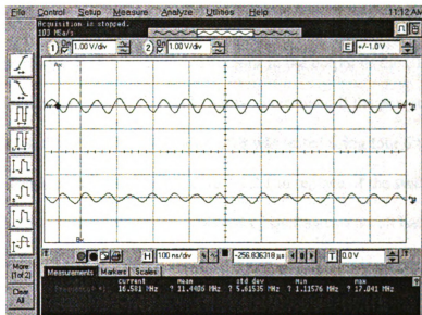
Figure 5.3.1.4: Plot of +/- 15 volt power supply pins - closer view
