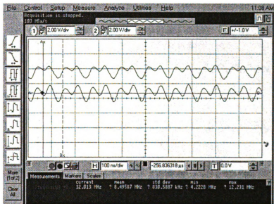
Figure 5.3.1.2: Plot of V_{OUT} and V_{OP-AMP} - closer view
