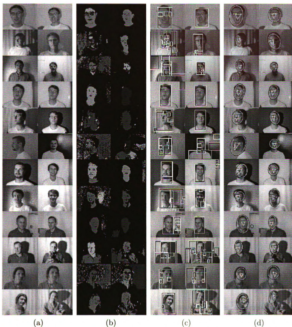
Figure 3.20. Face detection results on a subset of the HHI database: (a) input images; (b) grouped skin regions; (c) face candidates; (d) detected faces are overlaid on the lighting-compensated images.
