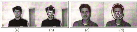
Figure 5.4. Face detection results: (a) and (c) are input face images of size 640 \times 480 from the MPEG7 content set; (b) and (d) are detected faces, each of which is described by an oval and a triangle.
