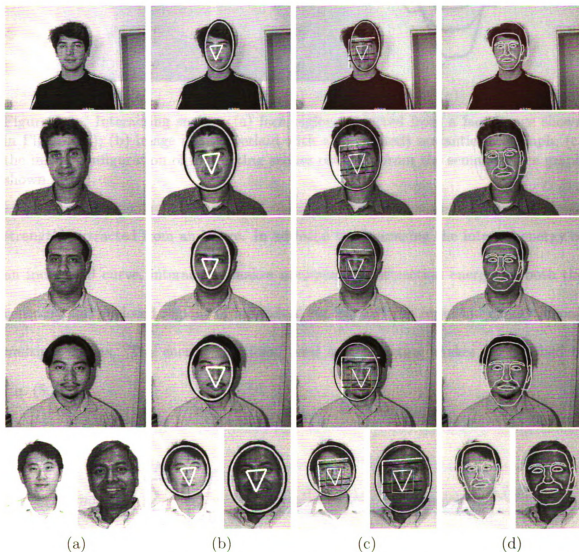
Figure 5.7. Coarse alignment: (a) input face images of size 640 \times 480 from the MPEG7 content set (first three rows), and of size 256 \times 384 from the MSU database (the fourth row); (b) detected faces; (c) locations of eyebrow, nostril, and mouth lines using shadow maps; (d) face images overlaid with coarsely aligned face graphs.
