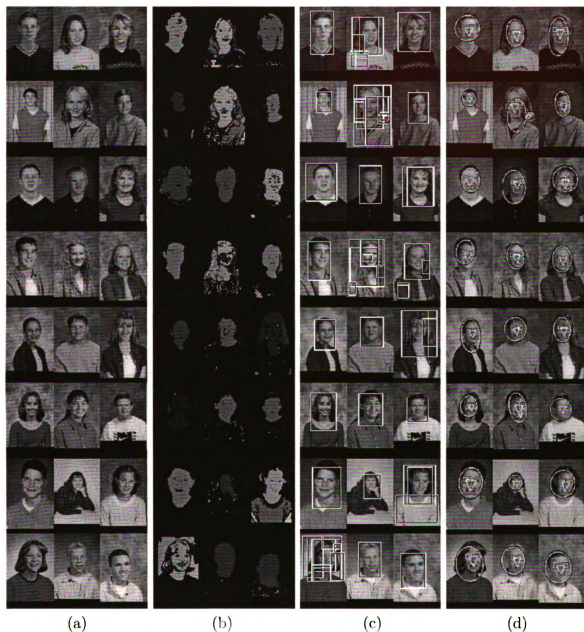
Figure 3.21. Face detection results on a subset of the Champion database: (a) input images; (b) grouped skin regions; (c) face candidates; (d) detected faces are overlaid on the lighting-compensated images.
