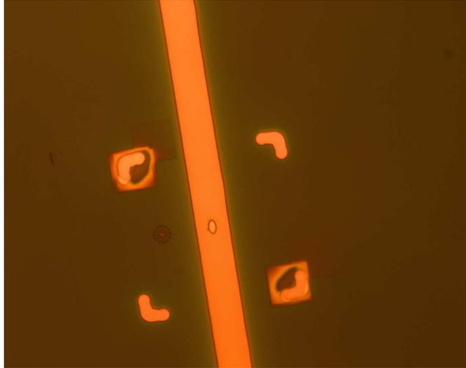
Figure 4.5: *Optical image of sample 2120 4A-2, a 4  $\mu\text{m}$  by 2  $\mu\text{m}$  Elliptical Pillar defined by Electron Beam Lithography. Note the four L-shaped alignment marks, including the two that have been clearly exposed to the electron beam.*
