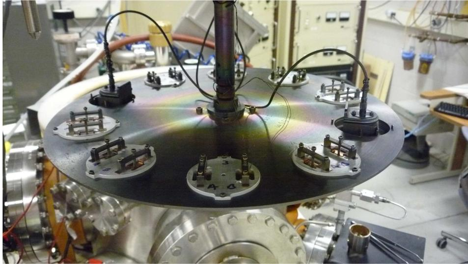
Figure 3.3: *The sputtering system SPAMA plate.* 8 sample holders have been loaded, each with two samples held down by bridges. To the right and left are the film thickness monitors.
