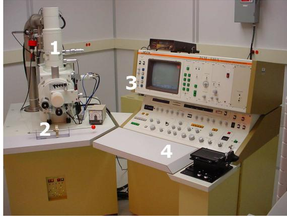
Figure 3.13: *The JEOL 840A.* 1) Electron beam column. 2) Sample exchange chamber and stage controls. 3) Display and controls. 4) Electron beam controls.
