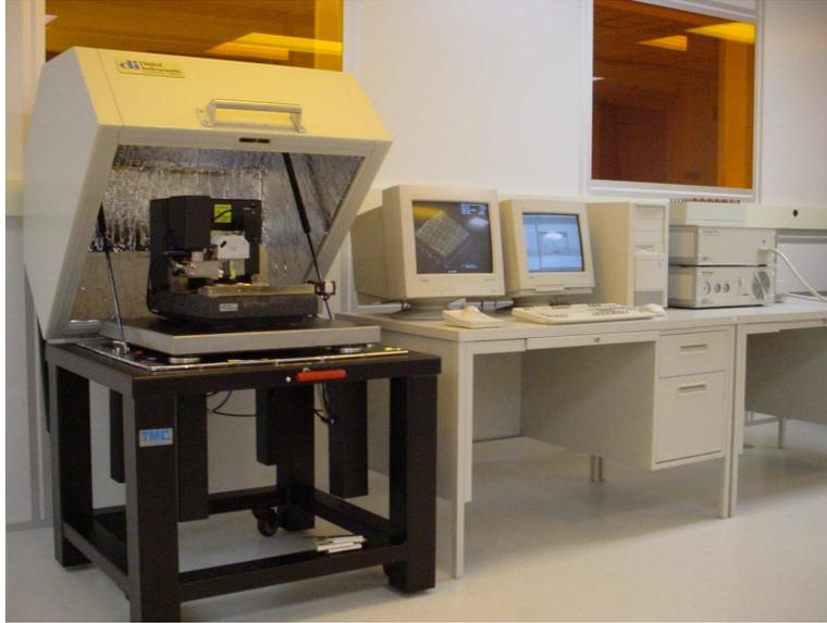
Figure 3.11: A picture of the Dimension AFM. From left to right are: the vibration isolated sample stage, the computer control station, and the Nanoscope control boxes.
