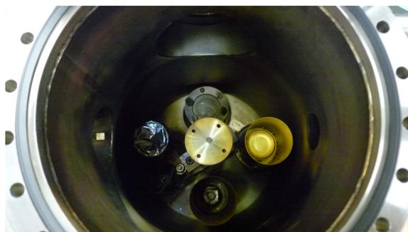
Figure 3.8: *Top view of the inside of the ion mill chamber.* North) The 3 cm ion mill. East) The 1.25" DC magnetron gun. South) The Silicon Monoxide evaporation source. West) Another gun that has been permanently disabled.
