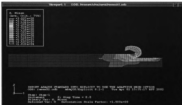
Figure 15: Chip Formation, Adaptive Meshing Applied
