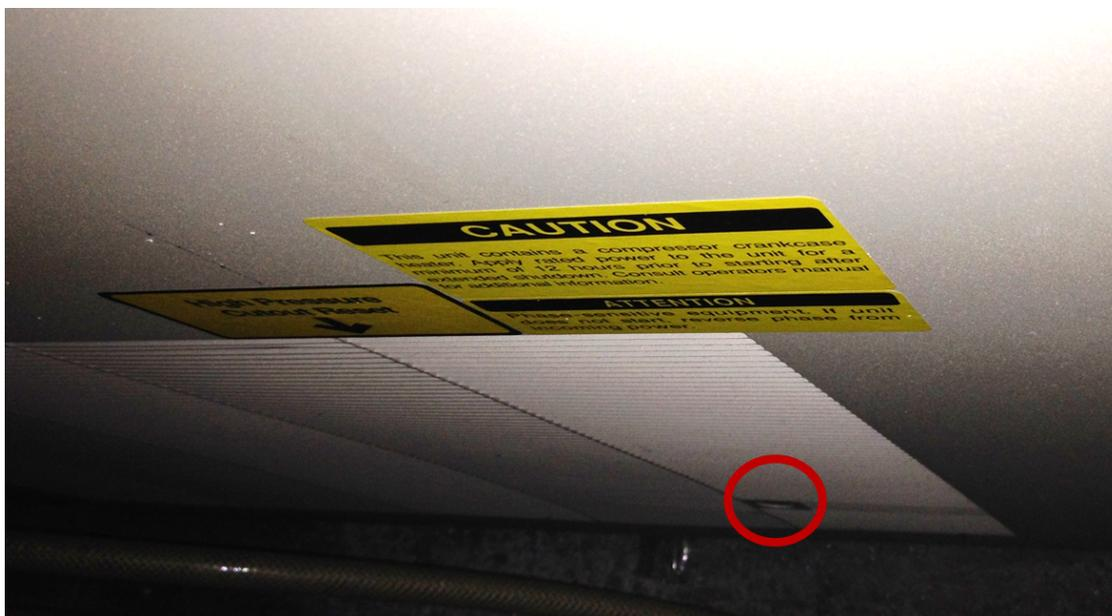
Figure 2.10 This photograph, taken looking down the back of the Neslab HX300, shows the location of the reset button, circled in red, that will clear the interlock that is triggered if the heat exchanger is run without sufficient water pressure from the house water line.
