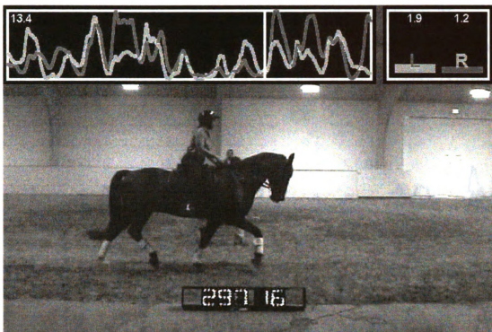
Figure 4.13 Video image with rein tension superimposed. On top left rein tension in the left rein (light line) and right rein (dark line) for a 5 second interval. White vertical line indicates time frame synchronized to video. At the top right of the picture left (L) and right (R) rein tension generated at that instant in pounds.
