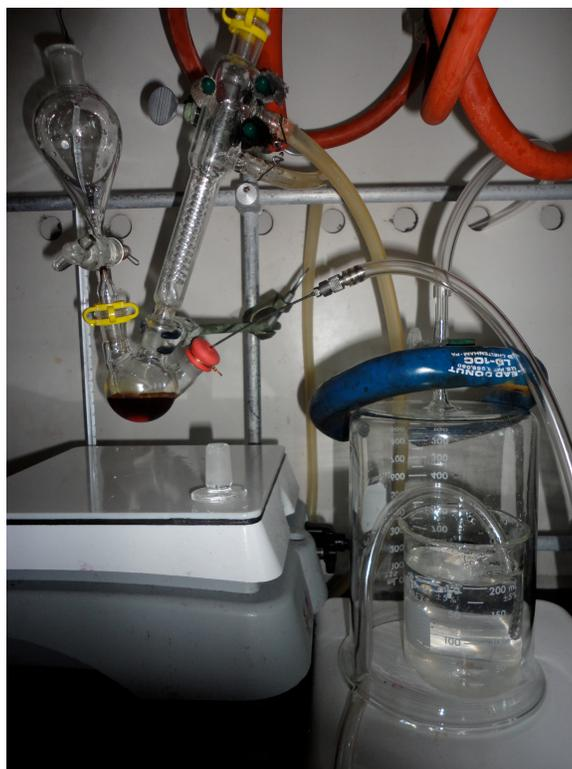
**Figure 3-19.** Setup for the reaction of  $\text{Ru(dcbpy)}_2\text{Cl}_2$  with  $\text{NaCN}$  to yield  $\text{RuCN}$ . The system is completely enclosed to ensure  $\text{HCN}$  containment. Acid addition is performed via a glass fitted separatory funnel attached to the reaction flask with a nitrogen inlet through the condenser and an outlet that bubbles through a basic solution.
