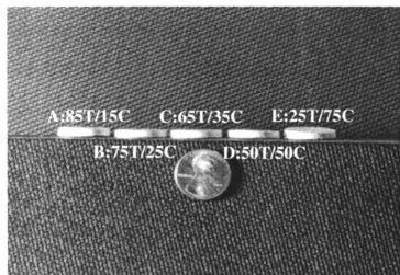
Figure 5.5: Five samples with two layers (alumina and zirconia mixed in five different ratios) showing varying degrees of warpage.
