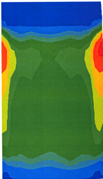
Figure 5.15b Shear stress contour (xz) for a traction at pressure of 100 psi, deflection of 48.9 mm (49613 N), friction of 0.95, v_t = 65 mph, v_r = 75 mph
