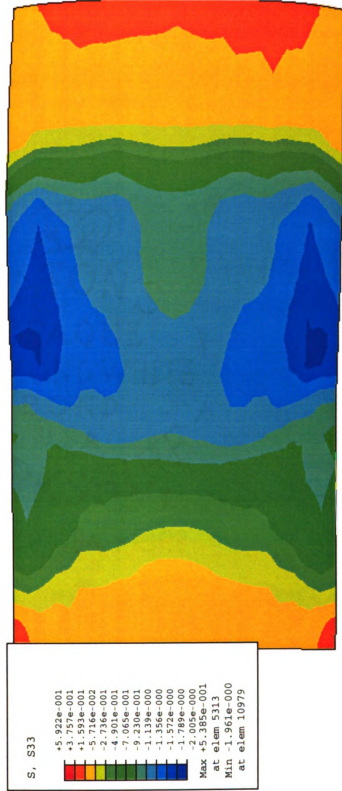
Figure 5.10a Normal stress contour for a braking at pressure of 90 psi, deflection of 49.6 mm (47797 N), friction of 0.95, v_t = 65 mph, v_r = 60 mph
