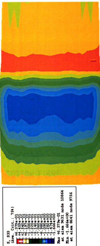
Figure 5.12a Normal stress contour for a traction at pressure of 100 psi, deflection of 29 mm (26414 N), friction of 0.95, v_t = 65 mph, v_r = 68.5 mph
