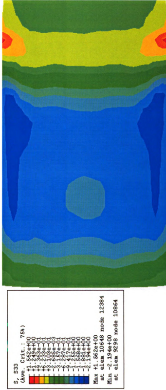
Figure 5.16a Normal stress contour for a traction at pressure of 110 psi, deflection of 48.4 mm (53372 N), friction of 0.95, v_i = 65 mph, v_r = 70 mph
