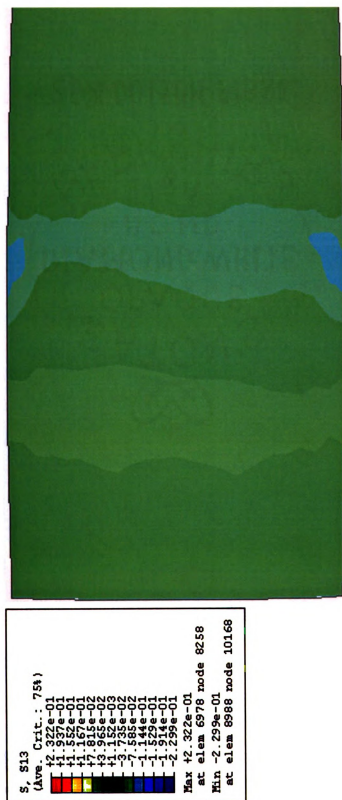
Figure 5.1b Shear stress contour (xz) for a free rolling at pressure of 90 psi, deflection of 22. mm (188871. N), friction of 0.95, and velocity of 5 mph
