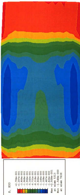
Figure 5.5a Normal stress contour for a free rolling at pressure of 100 psi, deflection of 48.9 mm (49613 N), friction of 0.95, and velocity of 45 mph
