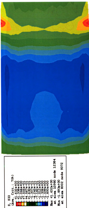
Figure 5.17b Shear stress contour (xz) for a traction at pressure of 110 psi, deflection of 48.4 mm (53372 N), friction of 0.95, v_t = 65 mph, v_r = 75 mph
