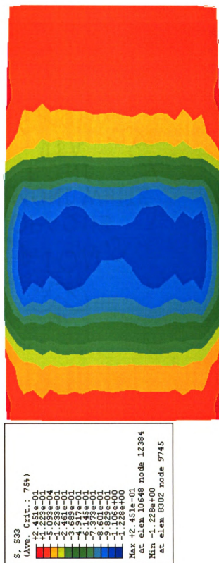
Figure 5.4a Normal stress contour for a free rolling at pressure of 100 psi, deflection of 29 mm (26414 N), friction of 0.95, and velocity of 65 mph
