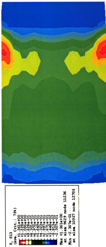
Figure 5.16b Shear stress contour (xz) for a traction at pressure of 110 psi, deflection of 48.4 mm (53372 N), friction of 0.95, v_t = 65 mph, v_r = 70 mph
