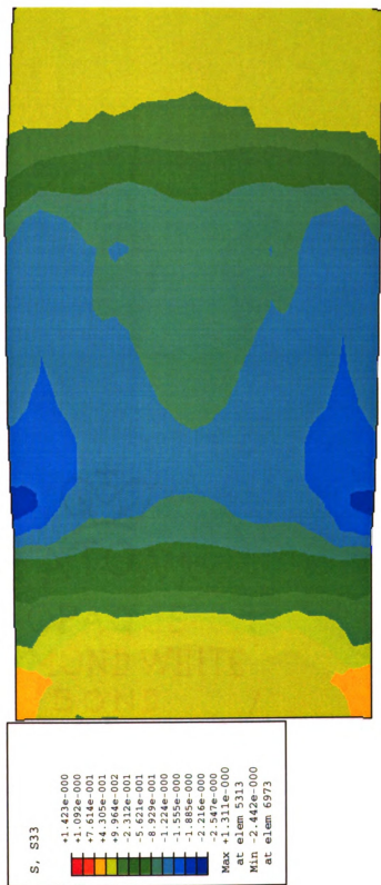
Figure 5.11a Normal stress contour for a braking at pressure of 90 psi, deflection of 49.6 mm (47797 N), friction of 0.95, v_i = 65 mph, v_r = 55 mph
