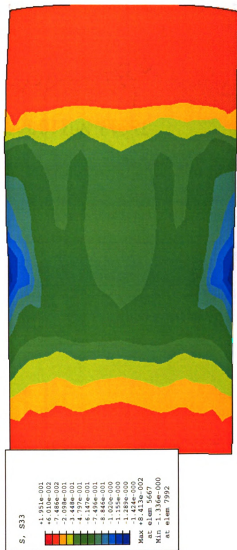
Figure 5.10b Shear stress contour (xz) for a braking at pressure of 90 psi, deflection of 49.6 mm (47797 N), friction of 0.95, v_t = 65 mph, v_r = 60 mph
