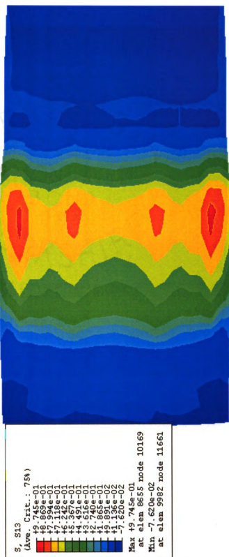
Figure 5.13b Shear stress contour (xz) for a traction at pressure of 100 psi, deflection of 29 mm (26414 N), friction of 0.95, v_i = 65 mph, v_r = 74.1 mph
