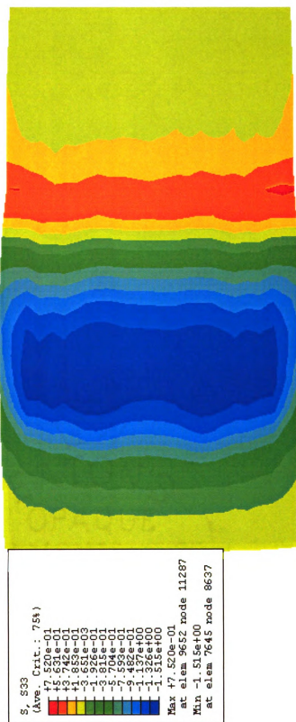
Figure 5.13a Normal stress contour for a traction at pressure of 100 psi, deflection of 29 mm (26414 N), friction of 0.95, v_t = 65 mph, v_r = 74.1 mph
