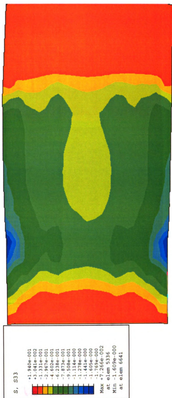
Figure 5.11b Shear stress contour (xz) for a braking at pressure of 90 psi, deflection of 49.6 mm (47797 N), friction of 0.95, v_t = 65 mph, v_r = 55 mph
