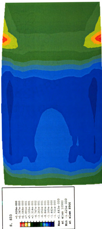
Figure 5.9a Normal stress contour for a traction at pressure of 90 psi, deflection of 49.6 mm (47797 N), friction of 0.95, v_t = 65 mph, v_r = 75 mph
