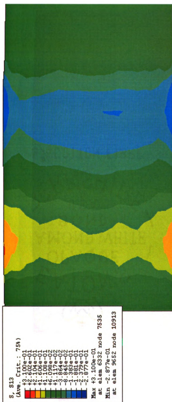
Figure 5.2b Shear stress contour (xz) for a free rolling at pressure of 90 psi, deflection of 42.2 mm (40000.0 N), friction of 0.95, and velocity of 5 mph
