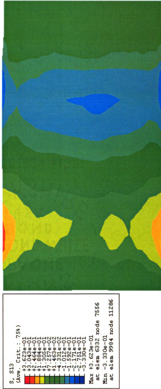
Figure 5.7b Shear stress contour (xz) for a free rolling at pressure of 110 psi, deflection of 48.4 mm (53372 N), friction of 0.95, and velocity of 65 mph
