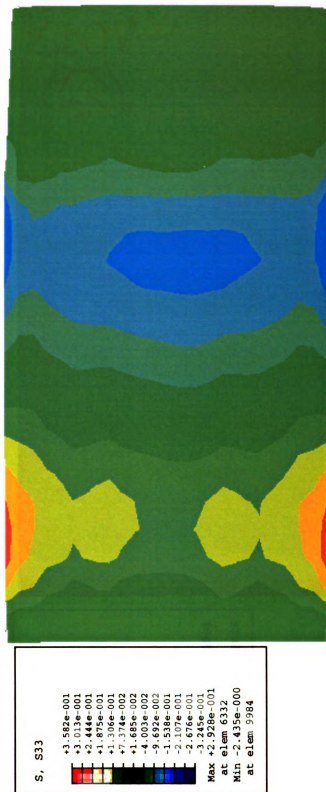
Figure 5.5b Shear stress contour (xz) for a free rolling at pressure of 100 psi, deflection of 48.9 mm (49613 N), friction of 0.95, and velocity of 45 mph
