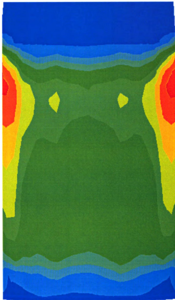
Figure 5.17a Normal stress contour for a traction at pressure of 110 psi, deflection of 48.4 mm (53372 N), friction of 0.95, v_t = 65 mph, v_r = 75 mph
