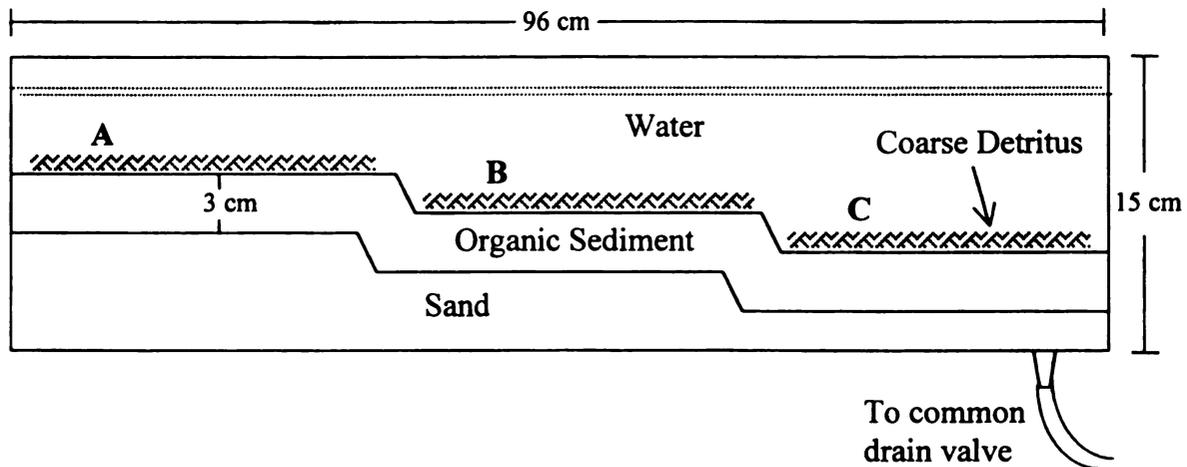
Figure 24. Diagram of the side view of one chamber in the Snail Movement experiment showing the arrangement of sand, sediment and water producing 3 tiers: shallow (A), medium (B), and deep (C). Initial water depth was adjusted so that water level was 4 cm above detritus. The drains of all 6 chambers were connected to one common valve used to maintain the same, constant reduction in water level. Width=42 cm.
