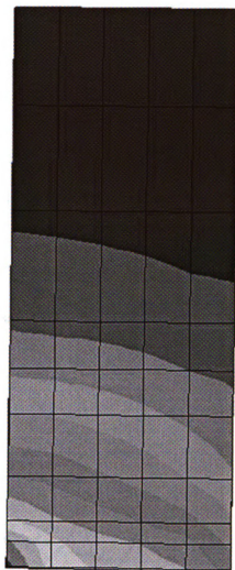
Figure 5.5 Distribution of shear stresses in the bearing plane of the resin plate for 4 in-lbs torque on the bolt and 120 lbs load on the joint (results are in psi).
