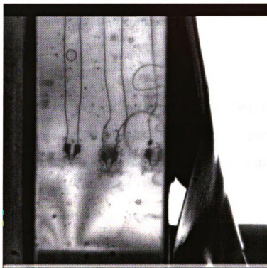
Figure 3.16. Shear stress fringe pattern in the bearing plane for a pin connection loaded at 50lbs.
