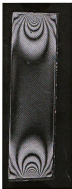
Figure 3.8. Fringe pattern in the specimen under compression load: a) one and a half fringe; b) two fringes; c) two and a half fringes; d) three fringes (all counted in the middle of the specimen)
