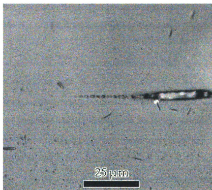
Figure 80 Higher magnification optical micrograph of one of the indent cracks shown in Figure 79. Extensive pinch-off at the end of the crack has occurred after annealing.
