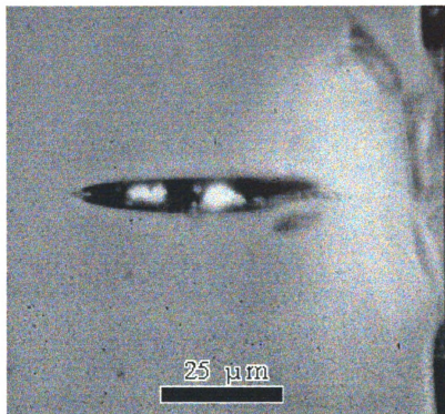
Figure 77 Higher magnification optical micrograph of one of the indent cracks shown in Figure 76. The crack tip appears blunted after annealing.
