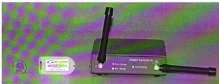
Figure 3.5: The RFID reader and tag used in our prototype system.
