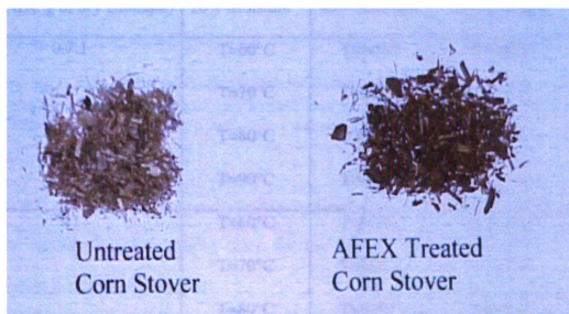
Figure 3.6. Physical appearance of AFEX treated and untreated corn stover.
