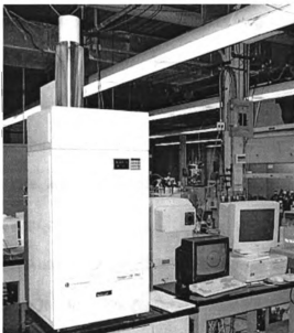
Figure 8.2: A MALDI MS similar to the instrument in our laboratory.
