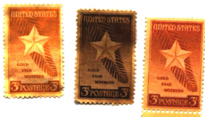
Figure 5.7: The Gold Star Mothers Stamps: a) Exposed to \text{H}_2\text{S} (g), followed by treatment with \text{H}_2\text{O}_2 (l); b) Exposed to \text{H}_2\text{S} (g); c) original (untreated).
