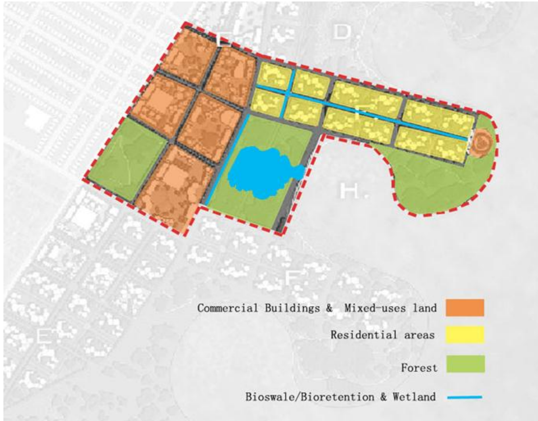
Figure 6. Locations of Bioswale/Bioretention and Constructed wetland.
