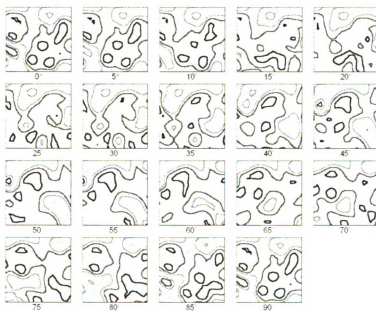
Figure 3-17b CODF representing the bulged 6061-T4 aluminum tube
