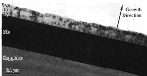
Figure 6.12 A cross-sectional brightfield CTEM image of the epitaxial (\text{Nb}_{200}/\text{Py}_{20}/\text{Cu}_{20}/\text{Nb}_{20})_{\text{nm}} multilayer with Py deposited at 150^{\circ}\text{C} on Nb showing the polycrystalline growth of the Py and Cu layers when Py grew on the Nb first instead of Cu.
