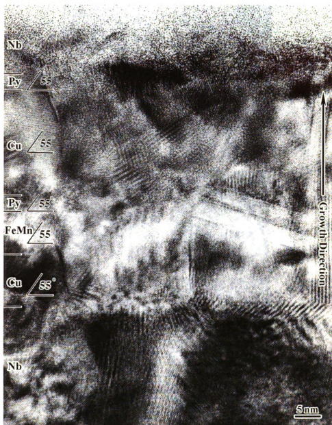
Figure 3.14 A cross-sectional HRTEM image of the [\text{Nb}/\text{Cu}_{10}/\text{FeMn}_8/\text{Py}_3/\text{Cu}_{20}/\text{Py}_3/\text{Nb}]_{\text{nm}} spin valve with 3 nm Py layers sputtered at 18^\circ\text{C} with nominal layer positions indicated. The individual layers of the spin valve are difficult to distinguish due to the small differences in the average atomic numbers of the multilayer components.
