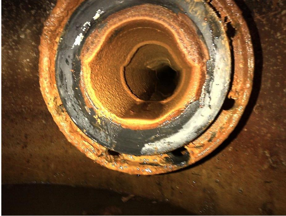
**Figure 1 - Mineral Scale in Pipe**
