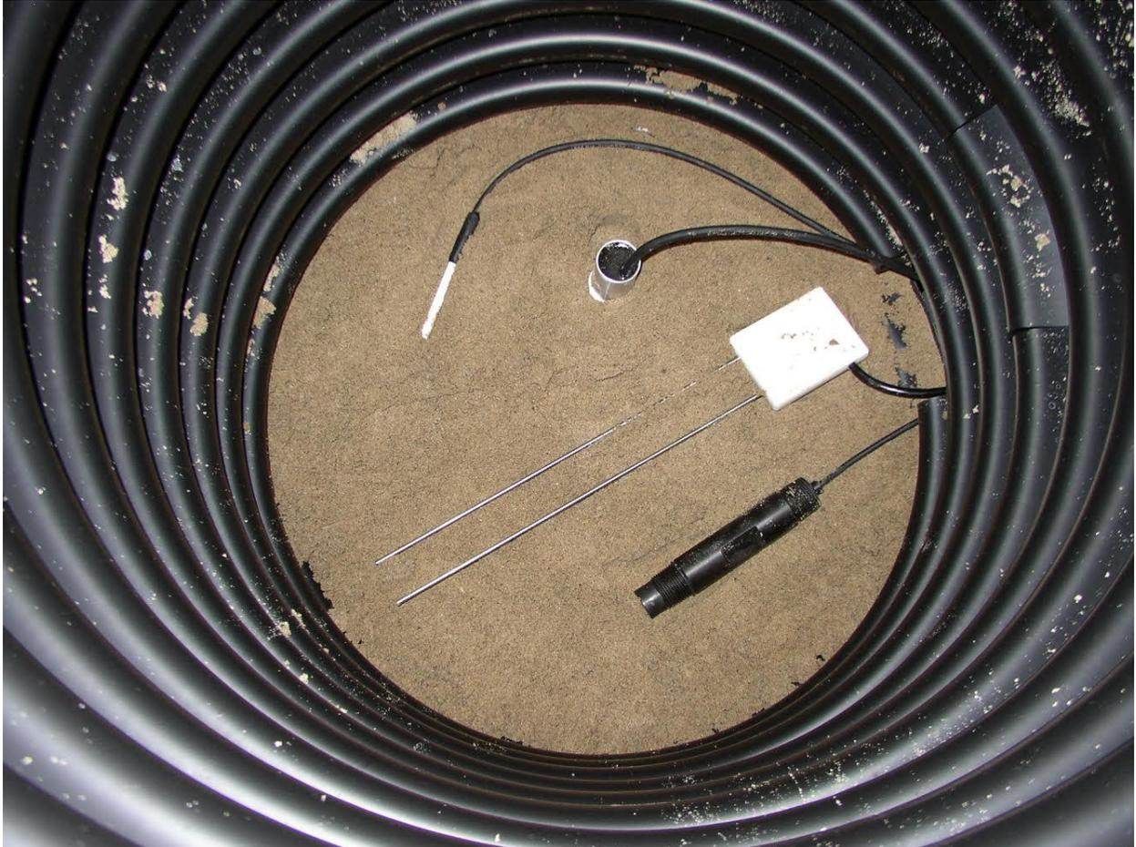
**Figure 3 - Sensor Placement During Column Construction**
