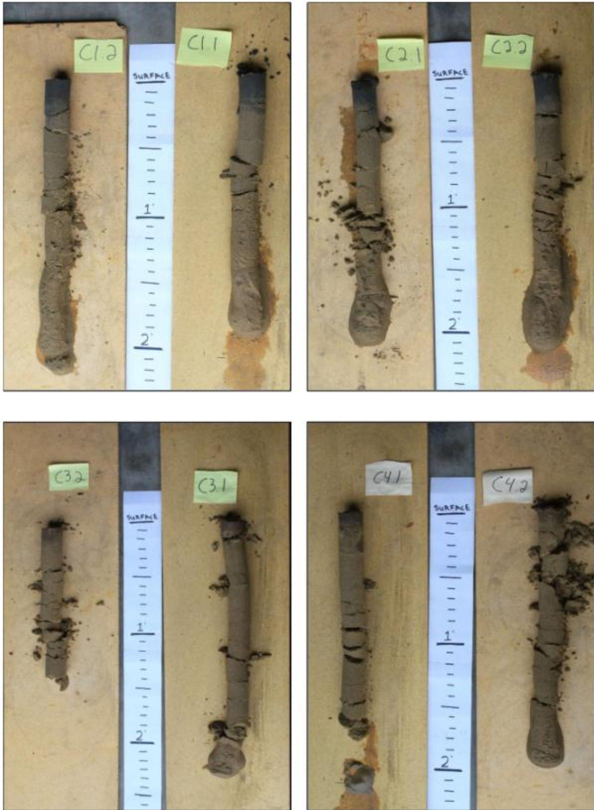
Figure 18 - Photos of Soil Cores from Columns One Through Four
