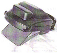
Figure 1.2: A prototype of the Head Mounted Projection Display.
