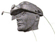
Figure 1.3: Complete integrated system of the head mounted display with the face capture unit.
