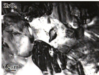
Figure 3.9 A TEM image of the microstructure of the zirconia in a joined 3 mol% yttria-zirconia/MaCor TM specimen at a location at about 10 μm away from the interface. The microstructure of the zirconia at this location is similar to that of the zirconia microstructure near the interface (Figure 3.6).
