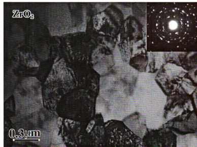
Figure 3.16 A TEM image of the bulk zirconia microstructure. The center of the image is about 5 \mu\text{m} away from the zirconia/MaCor TM interface. The diffraction pattern is consistent with a two phases partially stabilized zirconia structure.
