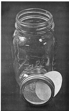
Figure 2.1. 0.5 L Mason jar used for rearing Galleria mellonella . Aluminum screen (1 mm openings) and 70 mm diameter Whatman no. 2 filter paper was placed in the outer ring of the Mason jar. The filter paper was used to prevent contamination and keep first and second instars from escaping from the jar. The wire screen was used to prevent larger larvae from escaping (third and fourth instars) from the jar.
