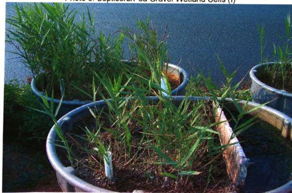
Photo 6: Septisorb/Pea Gravel Wetland Cells (Duplicate)
