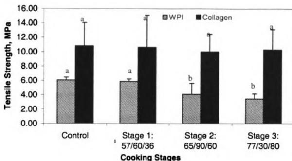
**Figure 2.4** Tensile strength of whey protein isolate based films heat-cured at 90°C for 12 hours and collagen films subjected to Polish sausage manufacturing conditions.  $n = 3$  for all treatments. WPI = whey protein isolate, control films did not undergo processing; <sup>a-b</sup>Different letters denote significant difference; cooking stage conditions: <sup>10</sup>C/min/%RH
