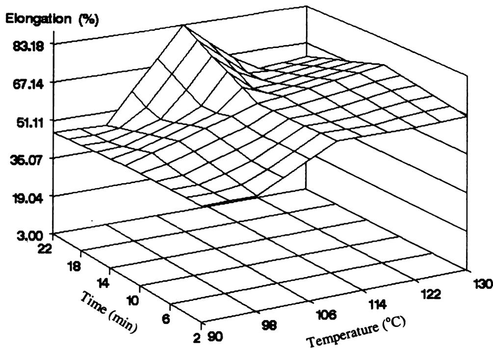
**Figure 3.7.** Effect of temperature and time on elongation (%) of 2-stage compression molded whey protein isolate-based films. Compression molding conditions: Stage 1: 110°C, 0.99 MPa, 25 min; Stage 2: 90, 98, 110, 121°C; 0.99, 1.10, 1.24, 1.38 MPa; 2, 12, 22 min. n = 3 for all treatments, No significant differences were found between treatment means.
