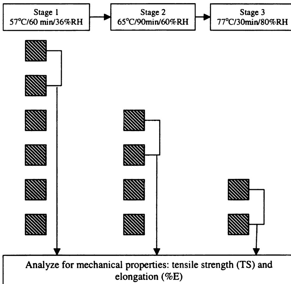
**Figure 2.2** Schematic diagram of meat processing simulation, each square represents a film sample. Stages 1, 2 and 3 represent sausage cooking stages.
