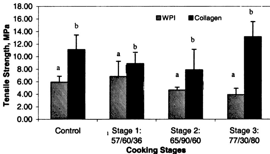
**Figure 2.3** Tensile strength of whey protein isolate based films heat-cured at 80°C for 24 hours and collagen films subjected to Polish sausage manufacturing conditions.  $n = 3$  for all treatments. WPI = whey protein isolate, control films did not undergo processing; <sup>a-b</sup>Different letters denote significant differences; cooking stage conditions: °C/min/%RH
