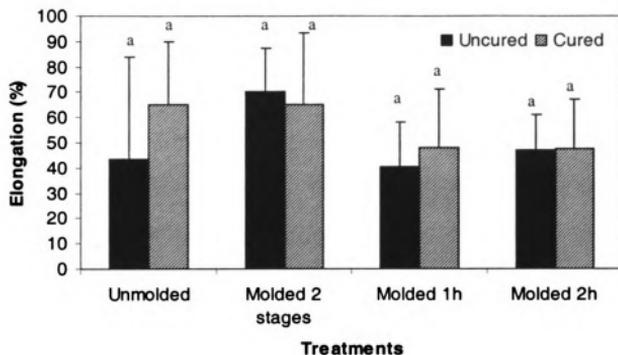
**Figure 3.3.** Elongation of compression molded whey protein isolate-based films. <sup>a</sup>Same letter denotes no significant differences between means; n = 3 for all treatments, Molded 2 stages = 2 stage molded: 110°C, 0.99 MPa, 25 minutes and 110°C, 1.24 MPa, 12 minutes, Molded 1h or 2h = single stage molded: 110°C, 1.24 MPa, 1 hour or 2 hours
