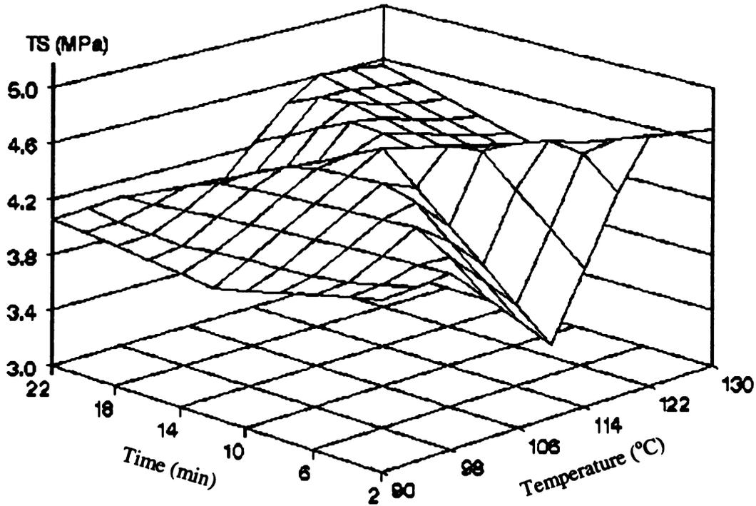
**Figure 3.5.** Effect of temperature and time on tensile strength (TS) of 2-stage compression molded whey protein isolate-based films as determined by response surface methodology.
