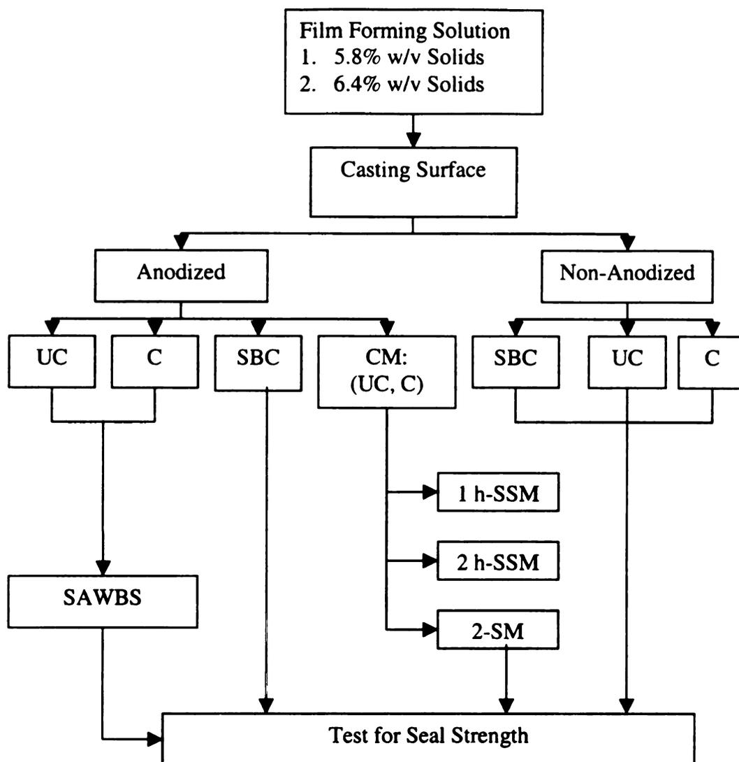
**Figure 4.1.** Schematic diagram of the seal optimization process for whey protein isolate based films
