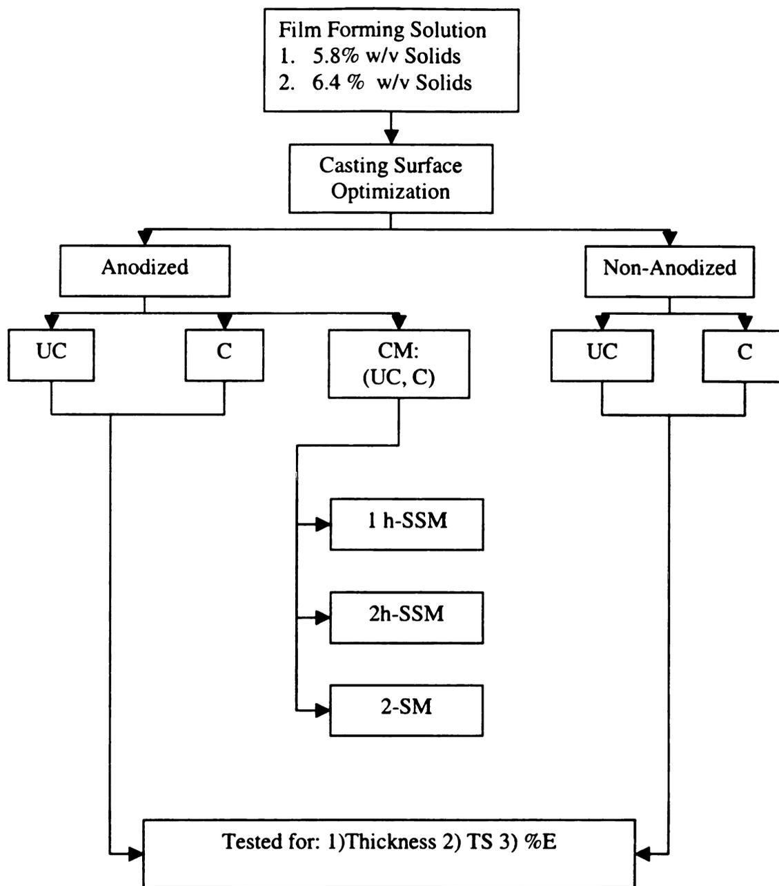
**Figure 3.1.** Schematic diagram of the film optimization process for whey protein isolate based films
