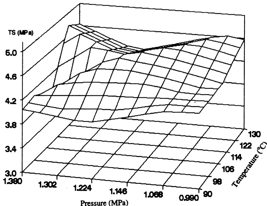
**Figure 3.4.** Effect of temperature and pressure on tensile strength (TS) of 2-stage compression molded whey protein isolate-based films as determined by response surface methodology.
