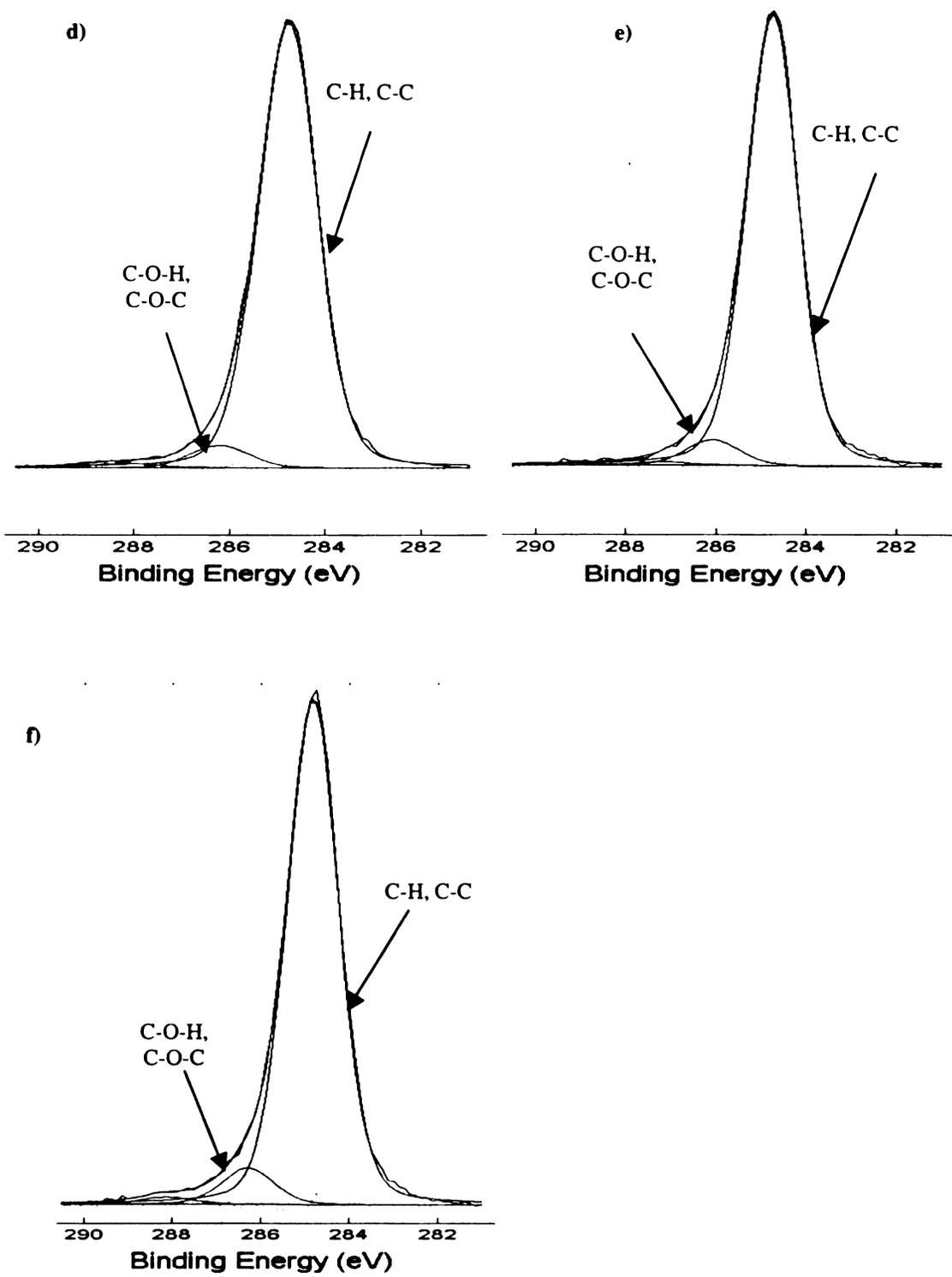
Figure 4.2b. Representative Electron Spectroscopy for Chemical Analysis spectra of whey protein isolate based films. d) cured e) cured outer seal f) cured inner seal
