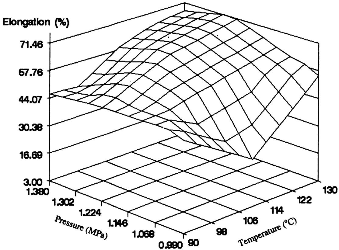
**Figure 3.6.** Effect of temperature and pressure on elongation (%) of 2-stage compression molded whey protein isolate-based films.
