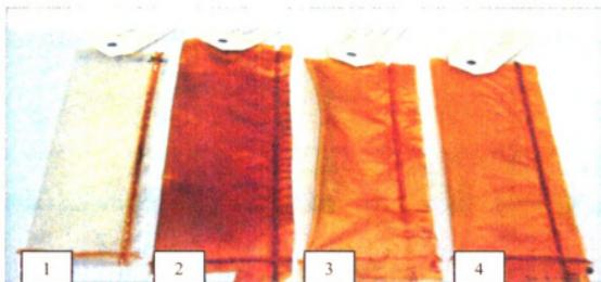
**Figure II.1.** Whey protein isolate based edible films heat-sealed to form sausage casings 1 = uncured film, 2 = compression molded film, 3 = film sealed before heat curing, 4 = heat cured film follows: pressure: 300kPa, voltage: 22 amps, impulse time: 1.8 seconds and dwell time: 1.4 seconds. Casings were made with uncured, heat cured and compression molded films
