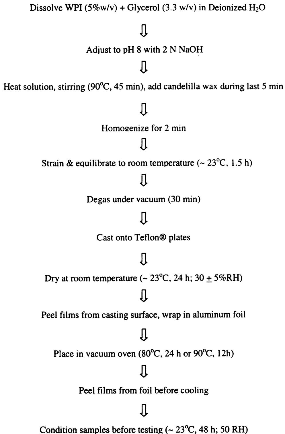
**Figure 2.1** Schematic diagram of film forming procedure
