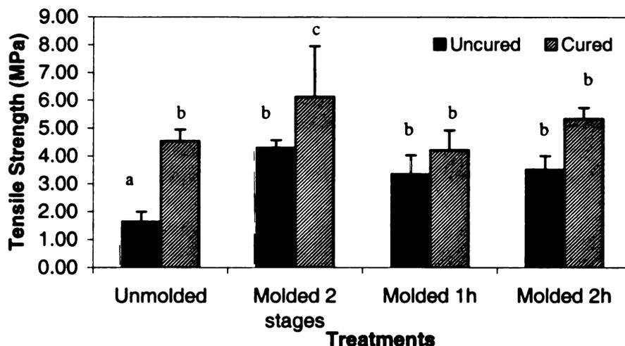
**Figure 3.2.** Tensile Strength of compression molded whey protein isolate based films. <sup>a-c</sup>Different letters denote significant differences;  $n = 3$  for all treatments; Molded 2 stages = 2 stage molding:  $110^{\circ}\text{C}$ , 0.99 MPa, 25 minutes and  $110^{\circ}\text{C}$ , 1.24 MPa, 12 minutes, Molded 1h or 2h = single stage molding:  $110^{\circ}\text{C}$ , 1.24 MPa, 1 or 2 hours
