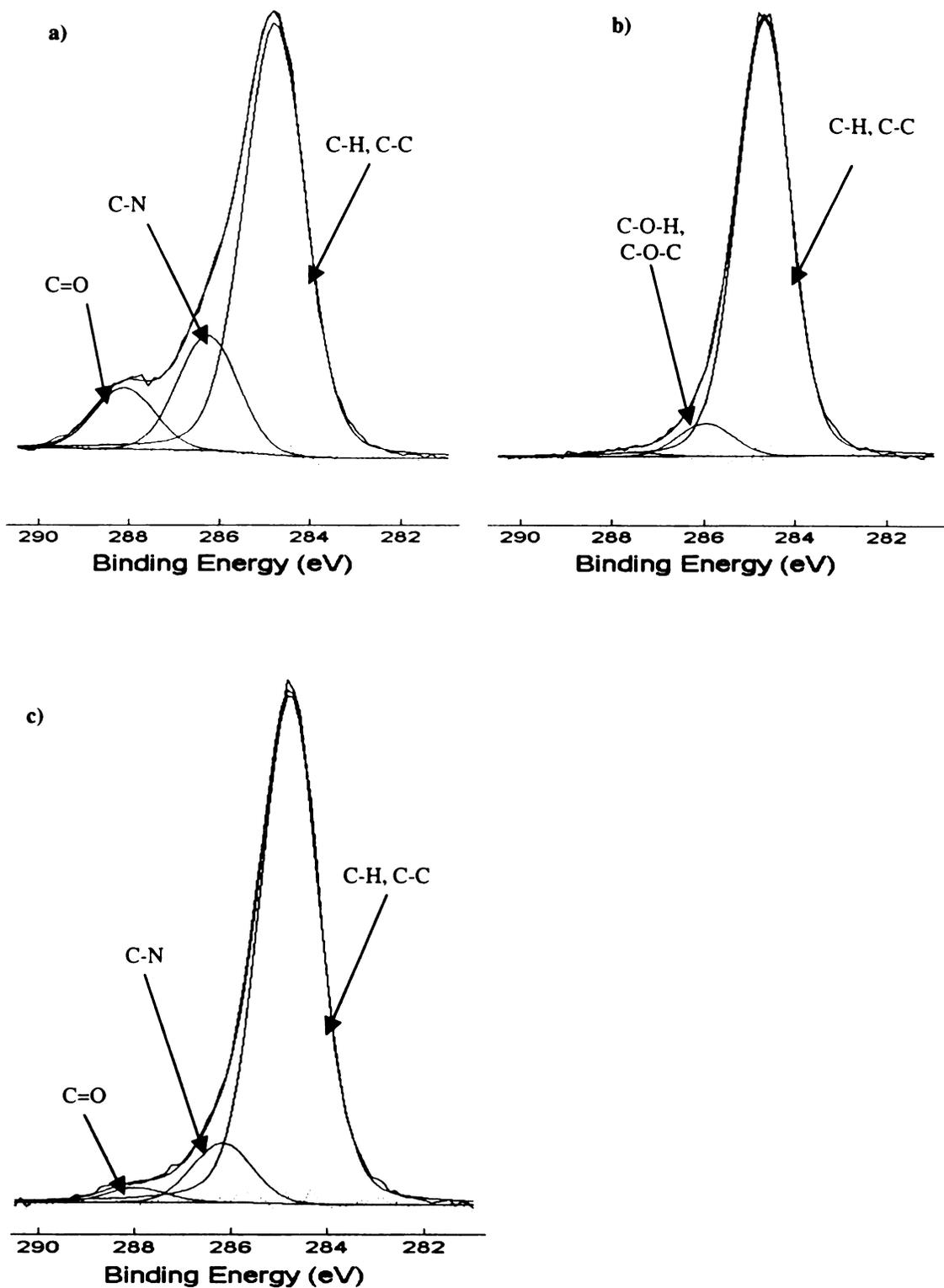
Figure 4.2a. Representative Electron Spectroscopy for Chemical Analysis spectra of whey protein isolate based films. a) uncured b) uncured outer seal c) uncured inner seal
