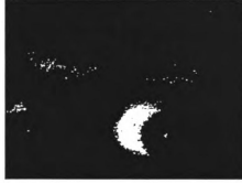
Figure 2.3: A binary difference image from two timely consecutive images.
