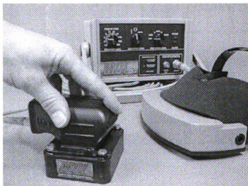
Figure 1.10: MOI system including handheld sensor (left), excitation unit (center), and wearable monitor (right).
