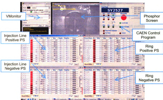
Figure 99: User interface of the video capture and high voltage power supply control programs.
