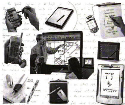
Figure 1.3: Devices that accept on-line handwritten data: From the top left, Pocket PC, CrossPad, Ink Link, Cell Phone, Smart Board, Tablet with display, Anoto pen, Wacom Tablet, Tablet PC.
