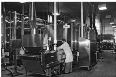
Figure 3.7 - Stein model JSO-IV moist-air impingement oven.
