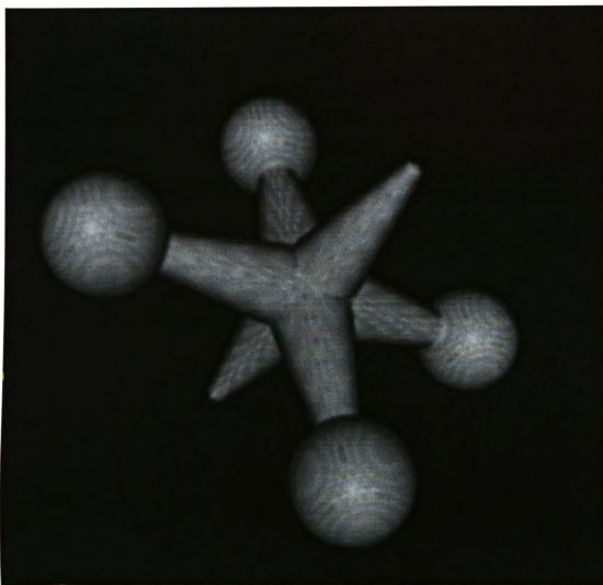
Figure 5.49: Rendering of jack phantom. The surface mottling is from the anti-aliasing used during phantom construction
