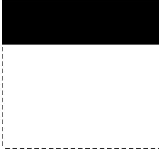
Figure 5.5 The reference flat design with a constant thickness of  $600\mu\text{m}$ , the black pixels represent the anode support; the white pixels represent the fuel flow path
