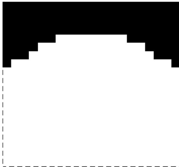
Figure 5.6 The optimal cross section in example 5.8.1 for the minimum probability problem
