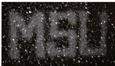
Figure A3 STM image ( 90 \times 120 \text{ nm}^2 ) of a H-passivated Si(001) surface. Brighter areas correspond to an STM-induced H desorption. By operating the tip position and the voltage, we can write a “MSU” logo!
