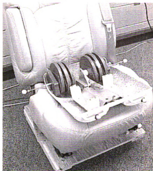
Figure 11: (Load step 5). Load step 4 plus two torso weights on H-pt axis just inside shell of ABT with a total weight 278 N. Front and Isometric views.
