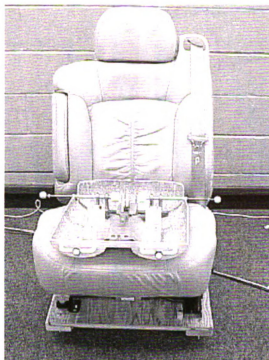
Figure 7: (Load step 1) Aspect Butt Thigh (ABT) segment with no weights added with a total weight 57 N.
