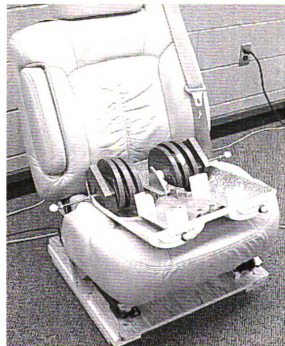
Figure 12: (Load step 6) Load step 5 plus two torso weights on H-pt axis just inside shell of ABT with slots down and back rear edge resting against shell with a total weight 310 N. Front and Isometric views.
