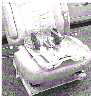
Figure 8: (Load step 2) ABT segment with two 6-plate H-point weights on H-point axes with a total weight 125 N. Front and isometric views.
