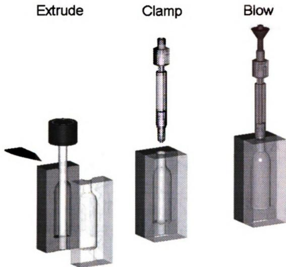
**Figure 3. Conventional Blow Pin**
