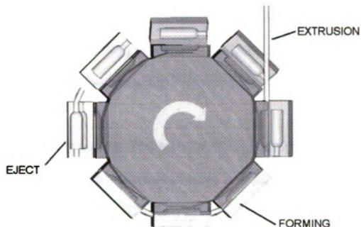
The wheel contains multiple molds and bottles are formed in each one. The wheel contains the air blowing mechanism, which punctures the parison to feed air inside. Rotary machinery is very expensive, due to the cost of the multiple molds and blow pins around the machine, but gives very high production rates. Rotary machines must produce millions of bottles to remain economical (Lee, 1990).
